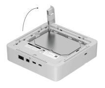
**4.** Install the hard drive in the NVR H enclosure so that the connectors match.
